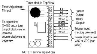
NOTE: Terminal legend can be found on back of PCB. †Relay rated 3A@24VDC
