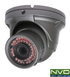
The EV-2646-NKGQ combines IR LEDs, Digital Noise Reduction (DNR), and a Digital Slow Shutter (DSS) that digitally slows the shutter 32 times its normal speed to capture a clear picture in total darkness.
