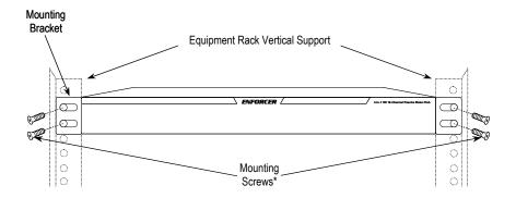
\*The screws included with the unit are for installing the mounting brackets. Screws for mounting the unit to an IT rack are not included.
