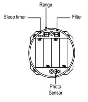
**c.** Filter – The detection speed of the sensor can be set for varying object speeds.
