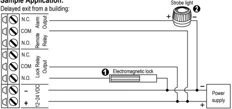
1. An electromagnetic lock, such as the E-941SA-1200, is connected to the lock relay output.
