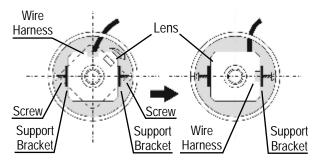
For wall mounting. Remove the 2 screws and turn the lens 90° clockwise until the wire harness is adjacent to the support bracket, then replace the 2 screws to secure it.
