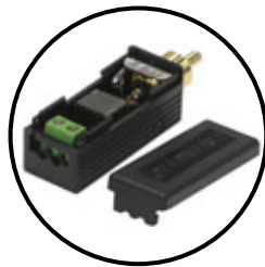
Figure 1 – Video balun with cover removed
