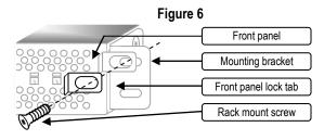
To close: Slide the lock tab toward the left over the front panel and tighten the screw.
